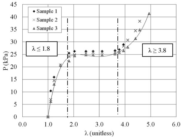
Figure 7 Inflation pressure and elongation ratio relationship for a latex membrane during bi-axial bubble inflation testing.
