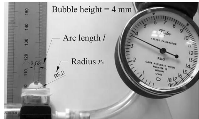
Figure 6 Graphic determination of the arc length  $l$  and radius of curvature  $r_c$  at a bubble height of 4 mm and corresponding inflation pressure of 25.51 kPa (3.7 psi).
