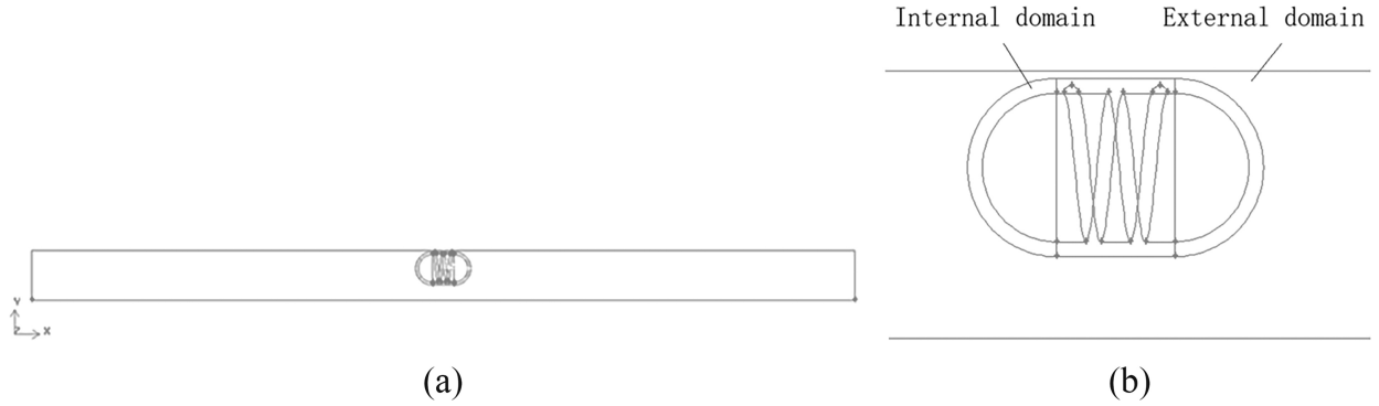
Figure 5. Computational domains of the fluid in the pipe for the capsule robot (No. 3): (a) overall view of the robot system and (b) enlarged view of the robot.
