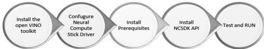
Figure 4. Steps involved in object detection on pi 3 with NCS.
