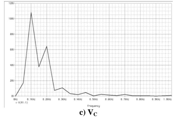
**Fig. 8. Three-phase voltage harmonics components**
