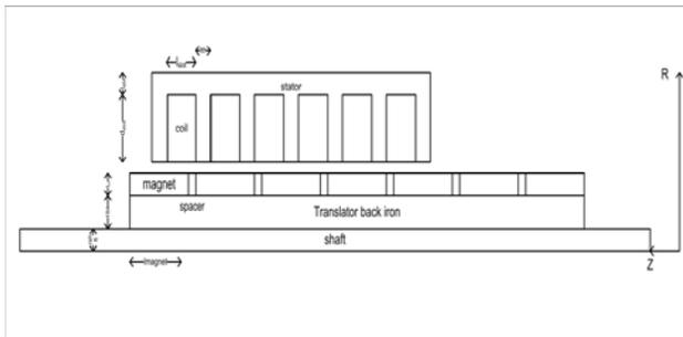
**Fig. 5. Three-phase linear generator modeling**
