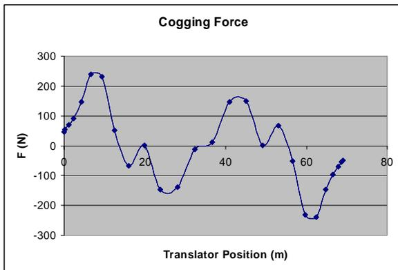
**Fig.7. Three-phase linear generator cogging force**
