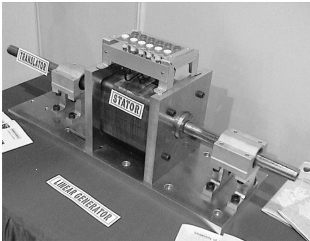
**Fig. 2. Three-phase linear generator**
