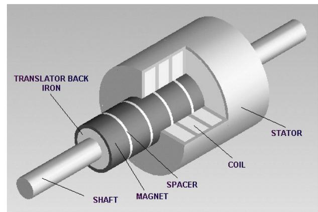
**Fig. 3. Three-phase linear generator components**
