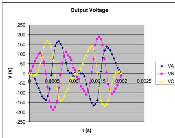
**Fig. 6. Three-phase linear generator output voltage**
