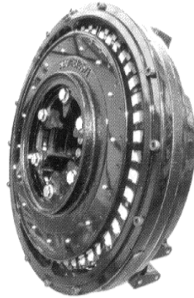
Fig. 7. Photograph of the Axial flux permanent magnet 40kW generator.
