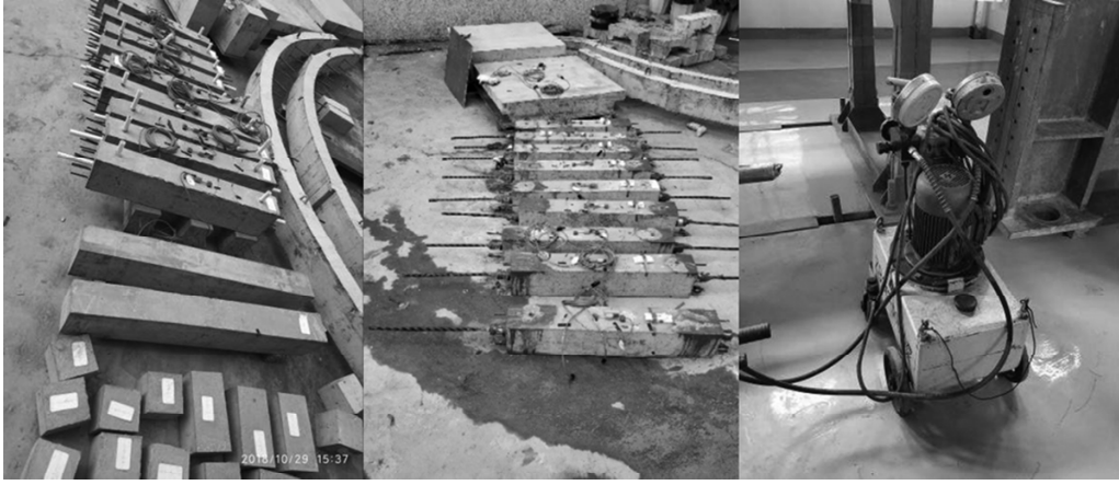
Figure 2. Test specimen and a pre-stressed tensioning device.
