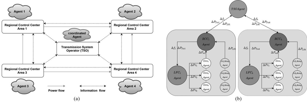
Figure 1. MAS representation of frequency control in multi-area power system: (a) frequency coordinated control; (b) frequency control in multi-area power system.
