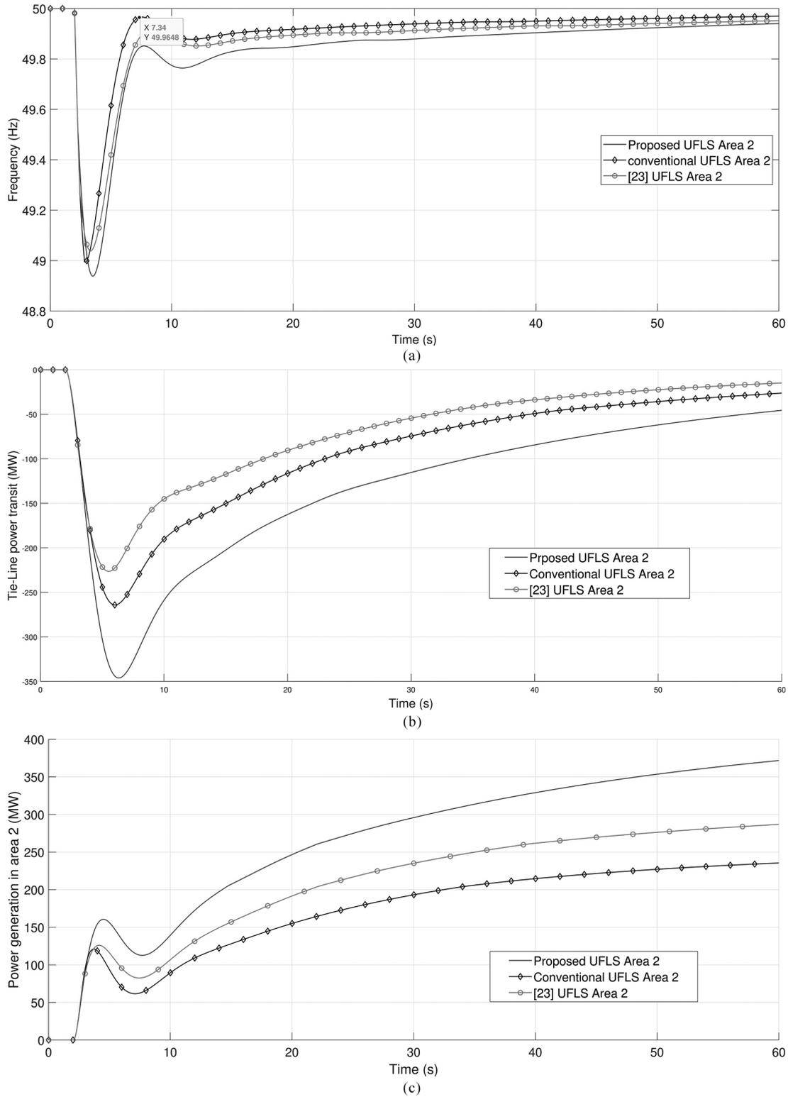
Figure 5. Frequency, tie-lines power transit, and spinning reserve in scenario 1: (a) frequency; (b) tie-lines power transit; (c) generated power in area 2.
