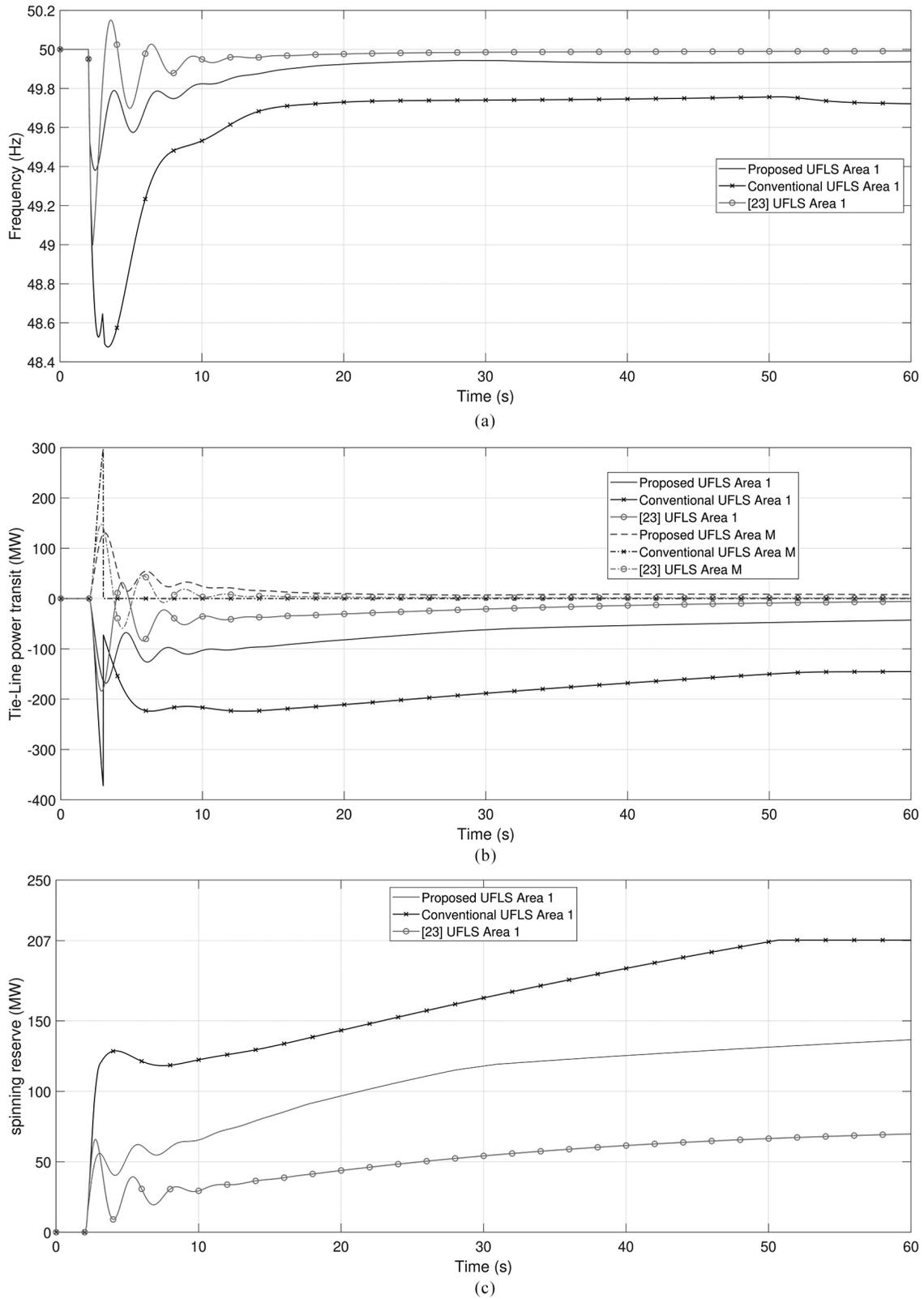
Figure 6. Frequency, tie-lines power transit, and spinning reserve in scenario 2: (a) frequency; (b) tie-lines power transit; (c) generated power in area 1.
