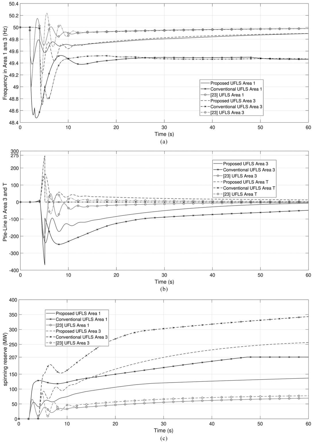
Figure 7. Frequency, tie-lines power transit and spinning reserve in scenario 3: (a) frequency; (b) tie-lines power transit; (c) generated power at area 1 & 3.
