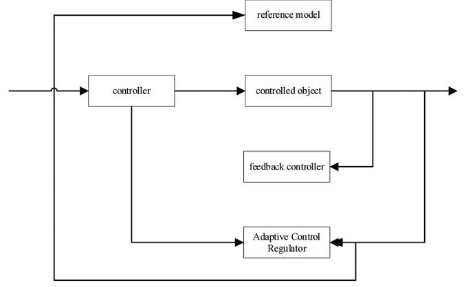
Figure 2. Model reference adaptive control.
