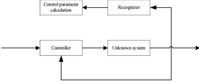
Figure 1. Automatic adjuster.
