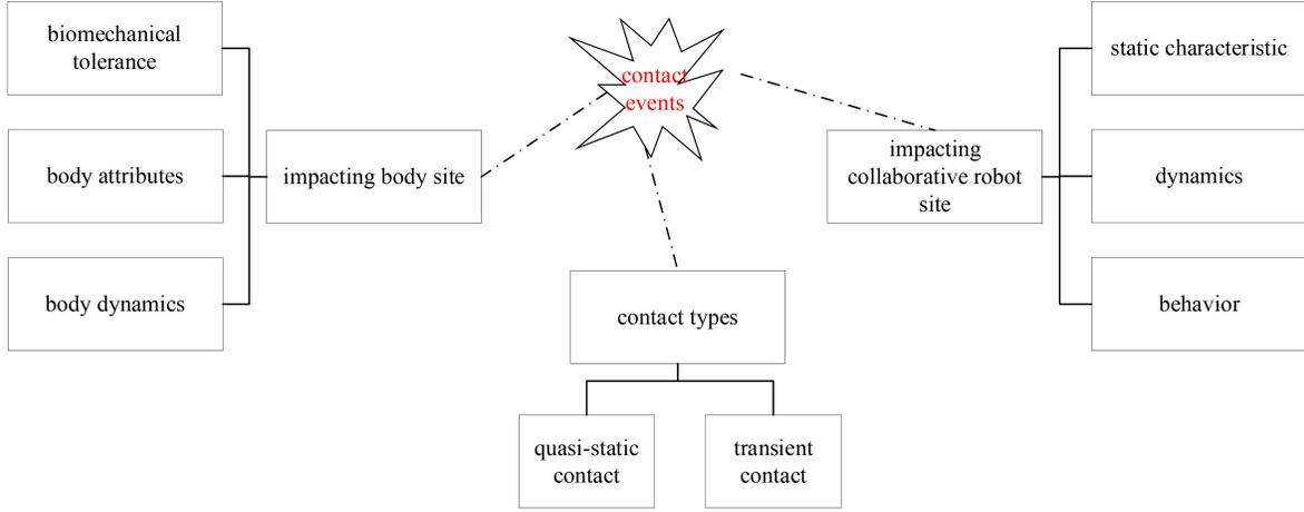
Figure 2. Aspects of human–robot collisions.
