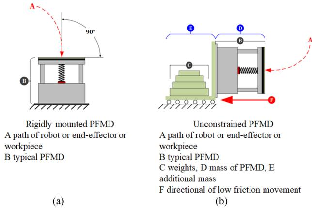
Figure 5. Installation of PFMD.
