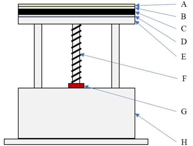
Figure 4. Typical PFMD representation. A – cloth, B – pressure sensing foil, C – damping material, D – teflon film, E – moving plate, F – spring, G – force sensor, H – base.
