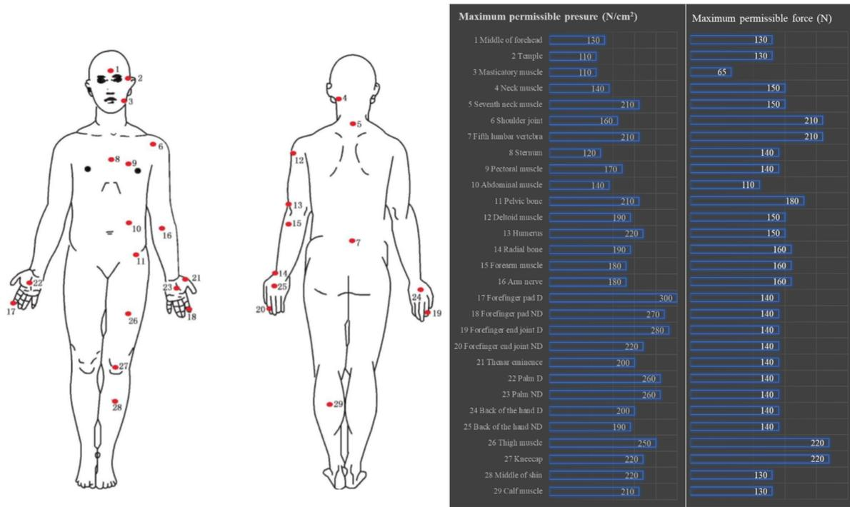
Figure 6. Body model and biomechanical limits in quasi-static contact.
