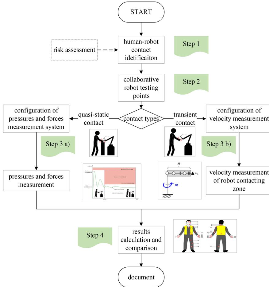
Figure 1. Collision safety assessment procedure.
