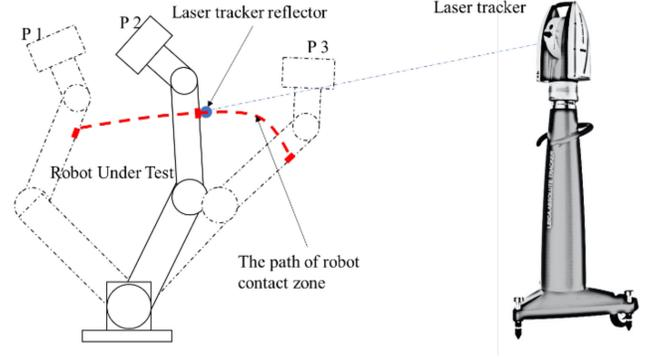
Figure 11. Velocity measurement of robot contacting zone.
