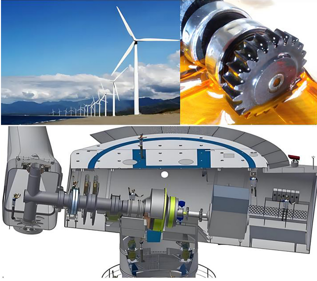
Figure 1. Schematic structure of wind turbine main gear system.
